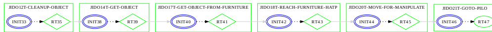
(a) Current execution task stack in SHARY: Boxes are tasks, circles and diamonds shapes are act_X_tasks (RT is the abbreviation of REALIZE-TASK), gray arrows represent decomposition links and dotted arrows are transitions between act_X_tasks inside a communication scheme. Blue color corresponds to achieved tasks and acts while green color means that they are being executed.
