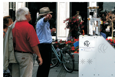
Figure 6. ACE following the pointing gesture of a passer-by with the camera head.
