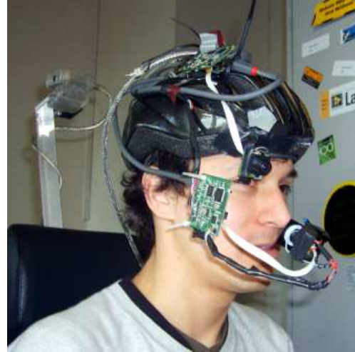
Figure 5. Our portable eye-tracker consists of two firewire cameras; one of which observes the subject's right eye, whilst the other records the scene (the person's field of view). After performing a manual calibration, the software will mark the person's focal point on the scene image.
