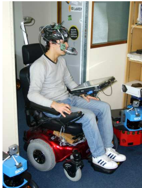
Figure 1. A participant driving our robotic wheelchair. The software on the tablet PC combines the stimulus from the joystick with the localisation data derived from the camera, to collaborate with the user in controlling the wheelchair motion. Simultaneously, the head-mounted eye-tracking system records the driver’s gaze.
