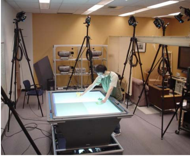
Figure 4. The user is holding two physical objects to interact with the virtual entities displayed on the SMART board. The board is surrounded with six Vicon motion tracking cameras for locating the reflective markers attached on top the objects to approximate their positions on the table.
