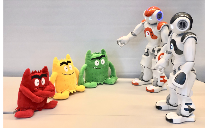
Figure 2: Two Nao robots play a grounded colour naming game with a scene consisting of coloured monsters. For each game, two agents from the population are physically instantiated in the two robot bodies.
